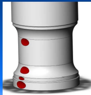
Common MRSE Damage Locations
