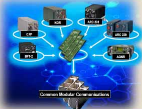
Convergence of RF LRUs & Waveforms into Single RF Chassis
